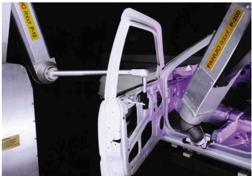
Typical robotic door cut-in applications.
